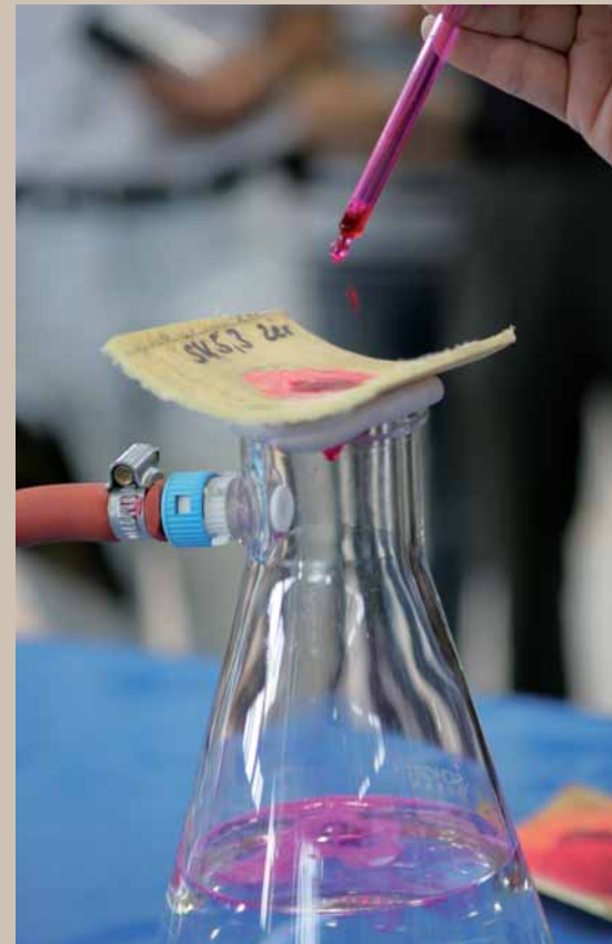
Figure 3: Water (stained red) permeates through: Liner is not water-tight
