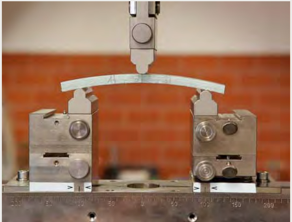
Figure 1: Liner sample undergoing the three-point bendig test
