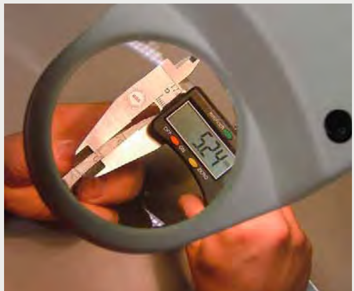
Figure 3: Measurement of liner-wall thickness
