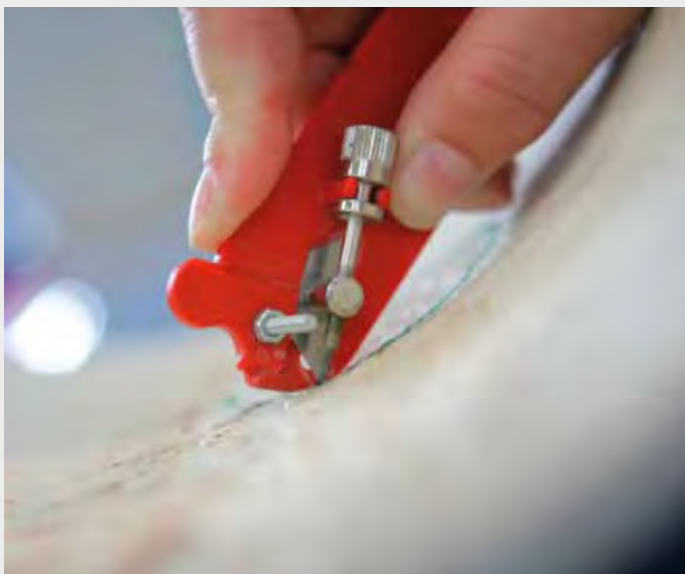
Figure 2: Cut made into inner film, with limitation of cut depth
