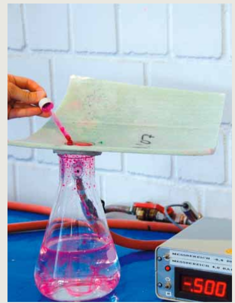
Leakage test: leaky liner
