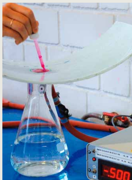
Leakage test: impermeable liner
