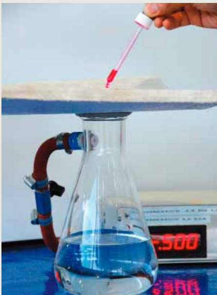
Leakage test: Red coloured water is applied to the inner side of the liner
